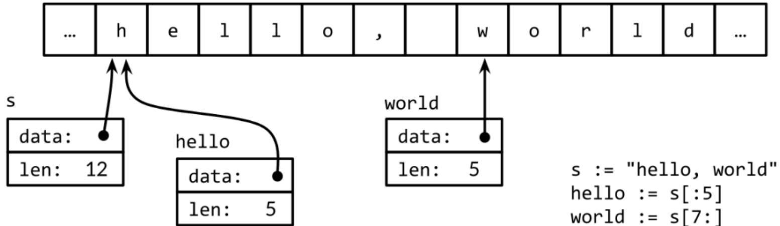
Figure 1: Memory layout of a string with substrings
