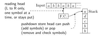
Transitions of PDA are of form  $(q, \sigma, \gamma) \mapsto (q', \gamma')$ , which means:
